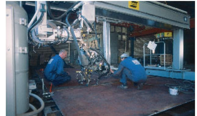
**Submerged Arc Welding ESAB 1250A**
